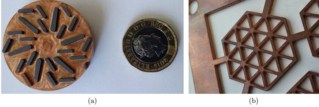
Figure 7.3: Machining methods investigated for HPJC-1b fabrication: (a) EDM electrode used to add channels to cascade plate and (b) waterjet cut triangular cavities.
