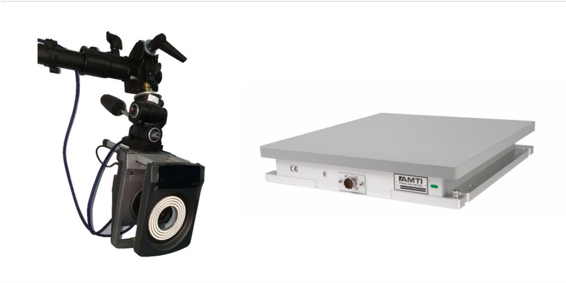
Figure 4.1: Vicon MX-T40 Camera (left) and AMTI OR6-6 force-plate (right).
