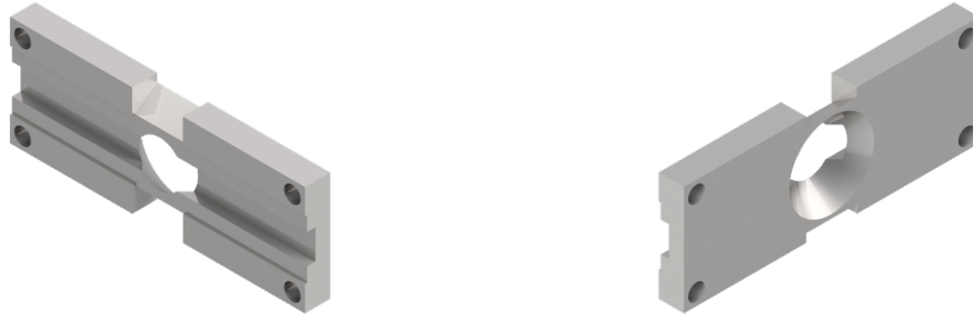
Figure 4.16: Cavity mount used to assemble the FFPC , showing the conical aperture to allow optical access for the focused tweezer beam. Recessed regions guide the shear piezos into the correct position. Screw holes at the corners allow us to implant it into the atom-cavity experiment; we discuss its implementation in section 5.2.1 .
