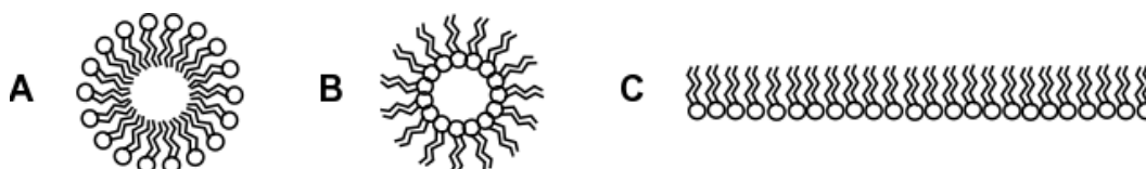
Figure 1.3: Selfassembly of lipids. (A) micelle, (B) inverse micelle and (C) a planar monolayer.
