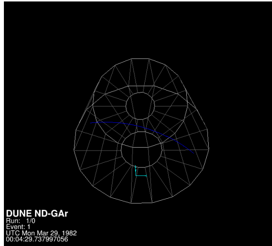
Figure 4.13: GArSoft event display showing a muon produced with the particle gun feature and used for the Lite-1 and Lite-2 studies. The layout of the tracker area is outlined in white and the trajectory of the muon is shown in blue.
