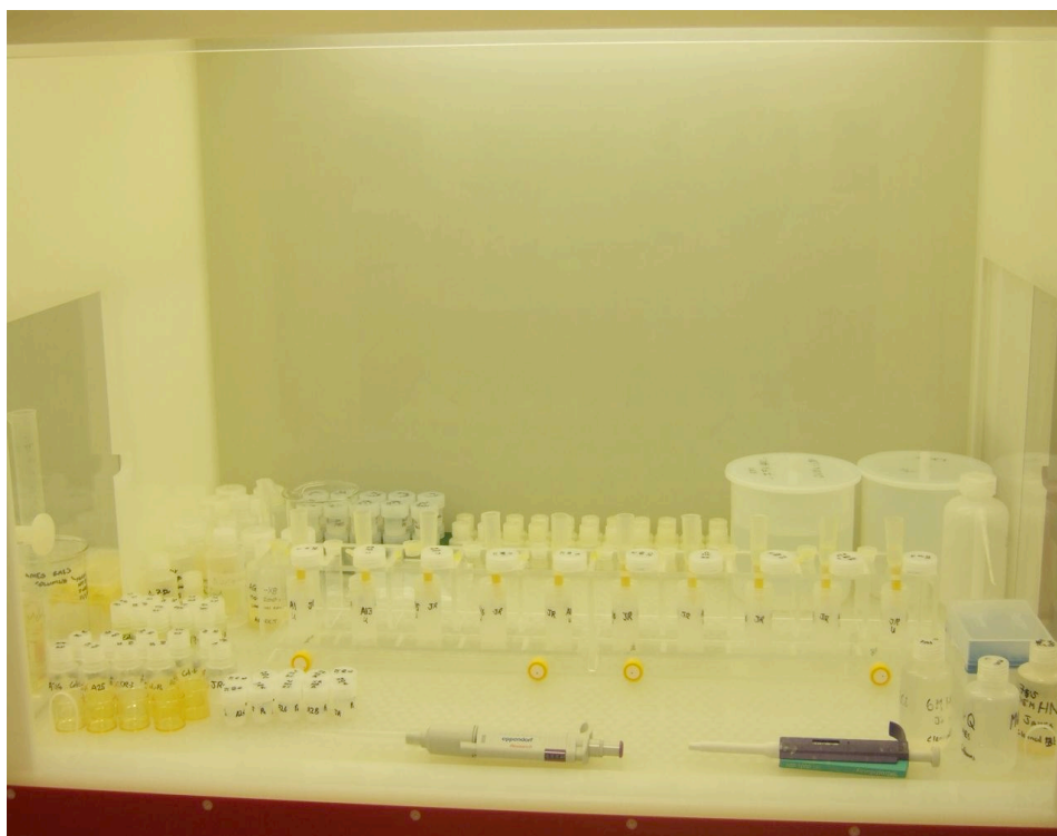
Figure 4.1: Photo showing laminar flow hood and materials used in column chemistry.
