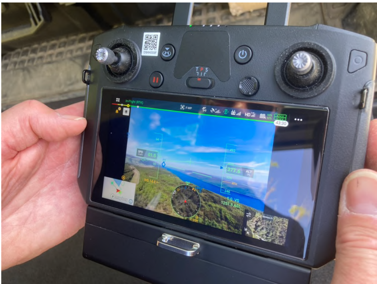
Figure 51 Eric's handheld remote for a drone-mounted camera, taking images of the forest canopy.
