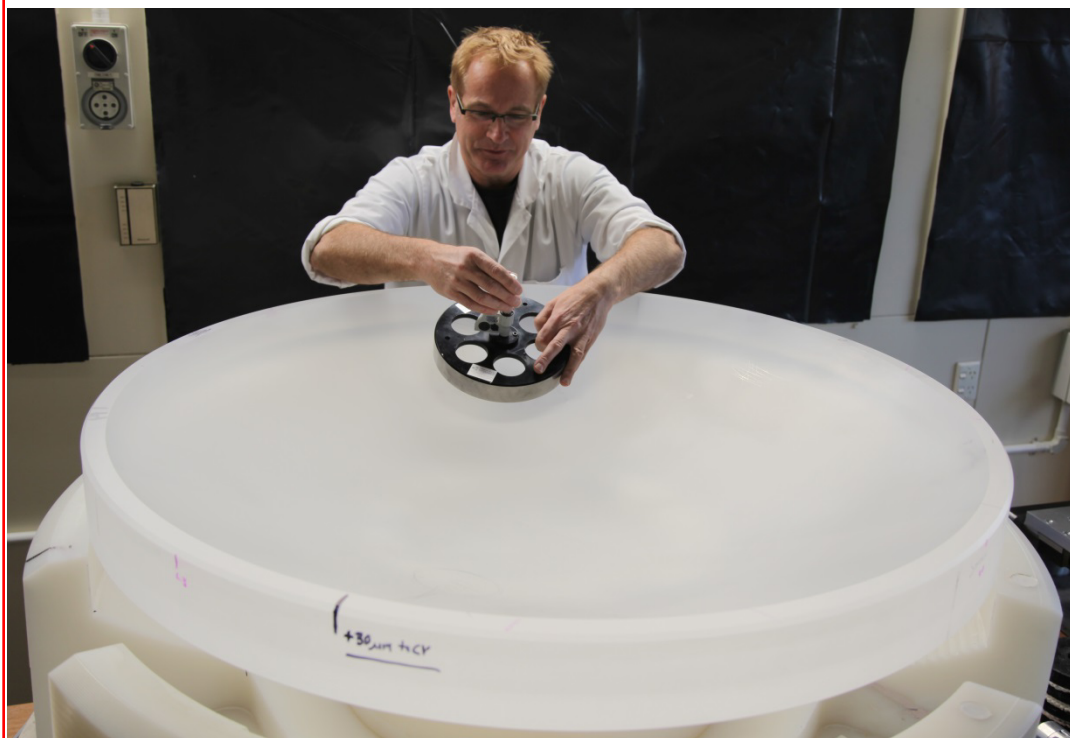
Figure 4: Verification of the geometrical dimensions of the lens concave surface on a Coordinate Measuring Machine. The blank is a 230kg meniscus of 1.1m diameter made of fused silica. The photo is courtesy of KiwiStar Optics.
