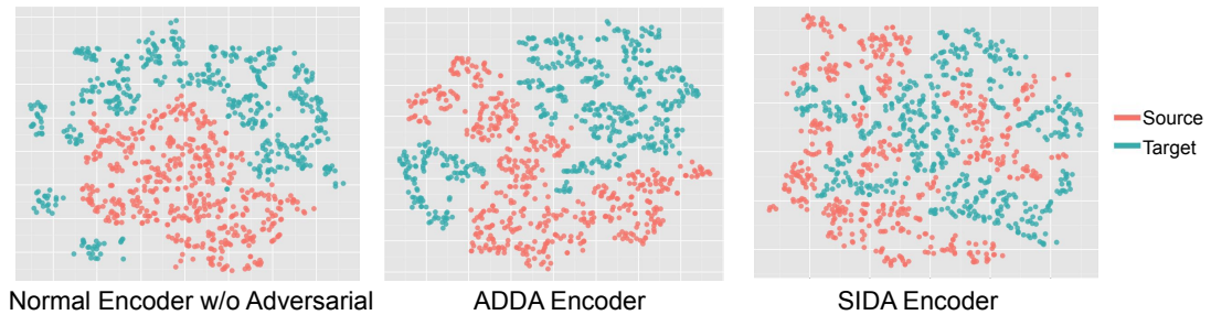
Figure 5.6: Visualization of extracted representations in the source and target domains by t-SNE. It can be seen that the SIDA leads to a more consistent latent representation compared with the disjoint representations of the normal encoder and the ADDA encoder.
