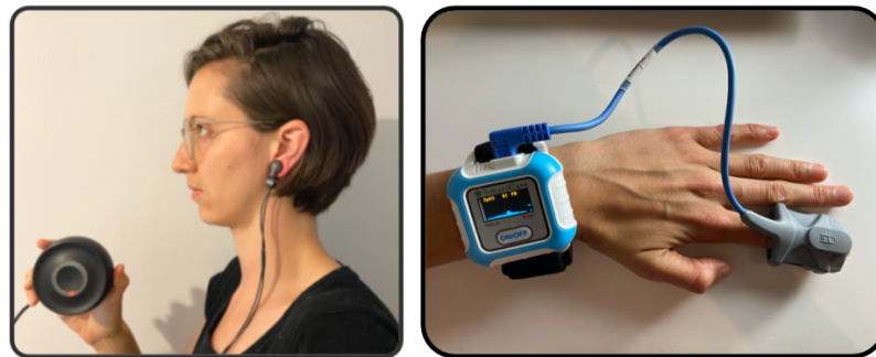
Figure 7.6: Low-cost wearable sensors used for collecting mobile physiological data from patients in limited-resource settings. PPG sensor with ear clip and storage-battery unit (left) and PPG sensor with a finger probe and display unit (connected to tablet or smart-phone via Bluetooth) (right).
