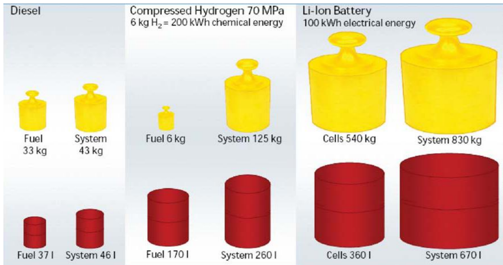
Figure 1.2. Comparison of a weight and volume specifications of different energy storage systems for mobile applications for equivalent driving ranges (18) (19).
