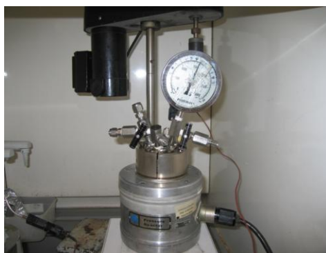
Figure 3.1. A Parr high pressure autoclave batch reactor used to carry out hydrogenation of 9-ethylcarbazole.
