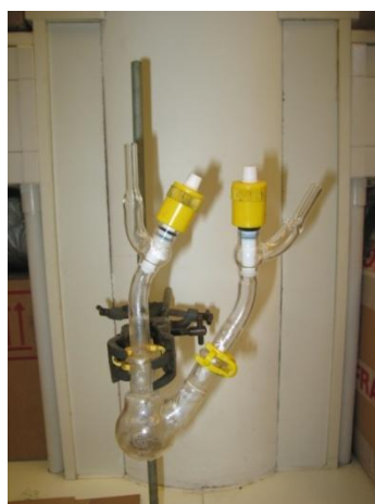
Figure 4.18. The set-up used for the dehydrogenation of the mixture of stereoisomers of 9-perhydroethylcarbazole over selected commercial catalysts.
