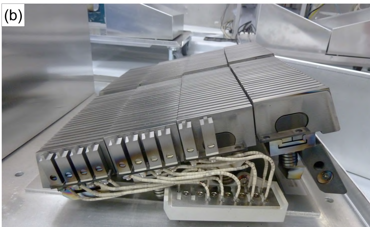
Figure 5.5: Digital photographs of a tile 5 module of lamellae (a) from a top-down view (b) from a cross-sectional view, showing the location of the tile 5 Langmuir probes.
