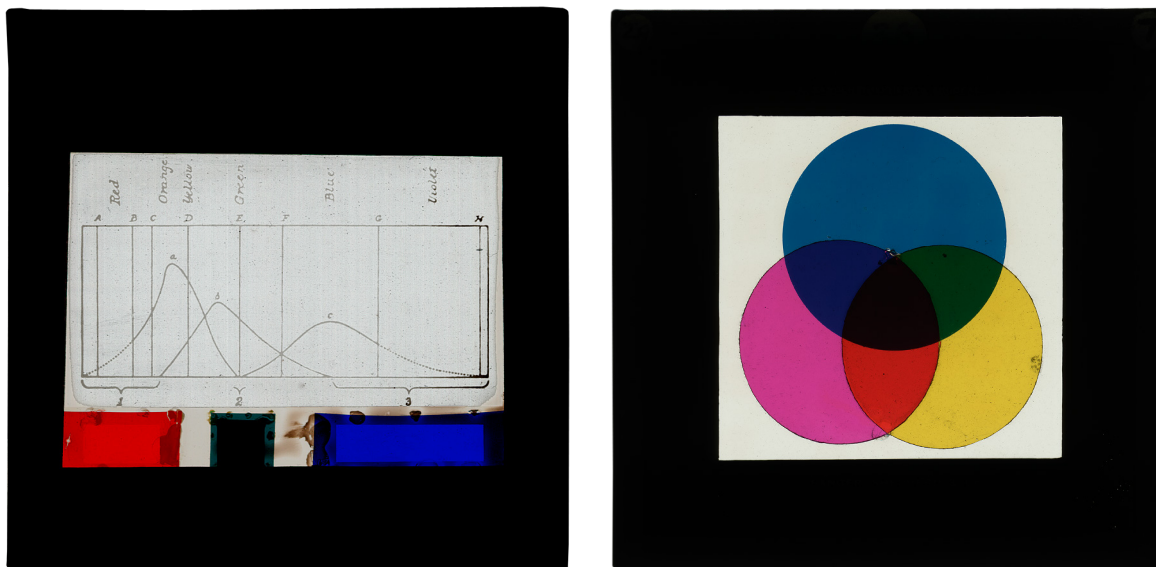
Figs. 6.2 & 6.3 [Sanger Shepherd & Co.], "Clerk Maxwell's Colour Sensation Curves"; "The Superposition of Red, Green and Blue Lights", lantern slides with coloured plastic overlays (MHS Inventory nos. 27920 & 28198)
