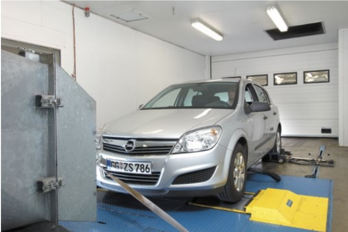
Figure D.8: The chassis dynamometer at Ricardo showing the rolling road.
