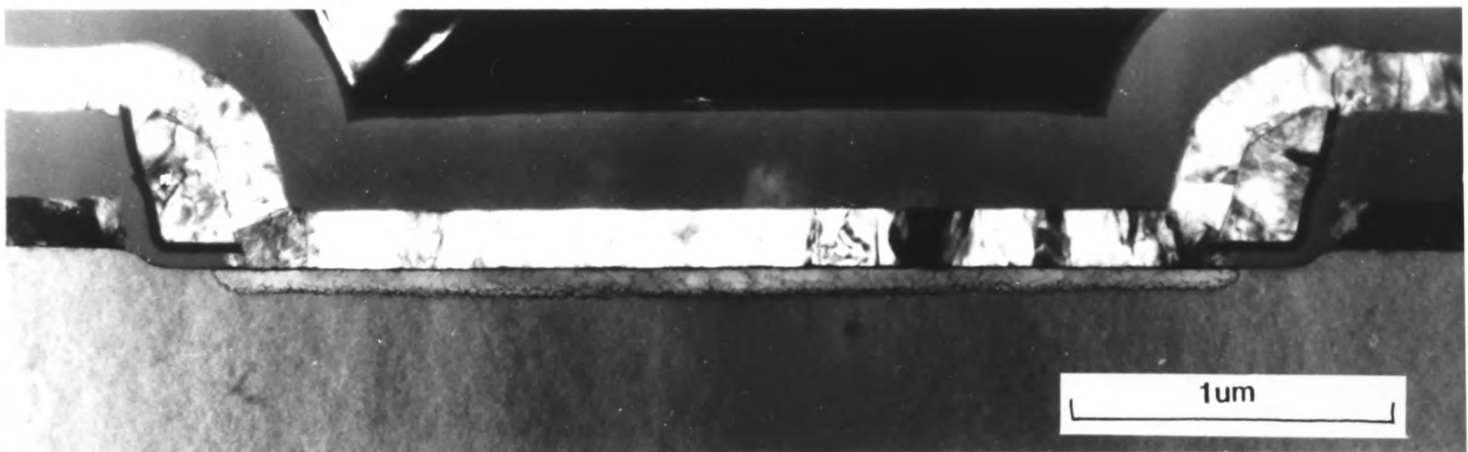
Fig.5.18b XTEM of Shallow Emitter
