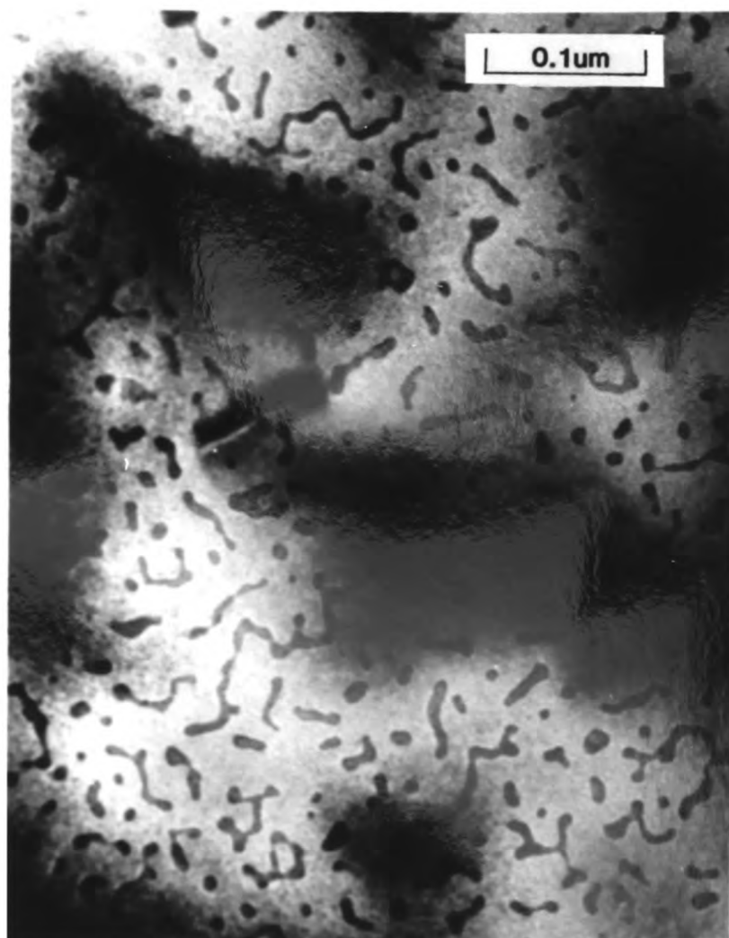
Fig.2.8a PVTEM of Broken Oxide Layer
