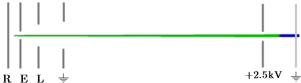
Figure 8.9: A diagram of the slicing apparatus designed to observe the pairwise correlations in the hexapole. The ion optics are the same as in the Townsend [243] DC slicing experiment. In the flight tube a set of inverting electrodes are used in order to stretch the Newton Sphere.
