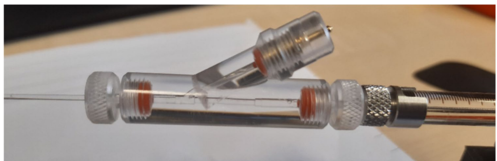
Fig. 4 Custom-made polycarbonate electrode holder with Ag/AgCl electrode placed in the arm of the holder. The holder is glued to the outflow syringe
