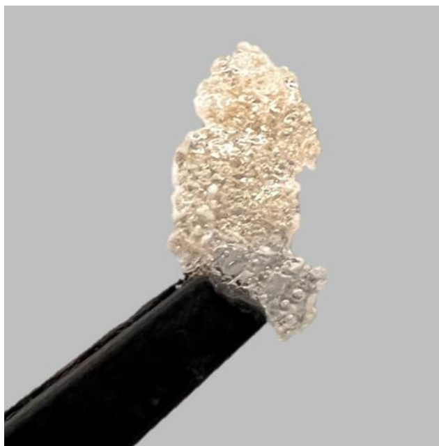
Figure 2.11: Actual photo of as-spun PMeABF heating to 300°C in NH 3 without curing process. Direct heating of PMeABF under NH 3 causes the fibers to melt and fail to retain fibrous morphology.
