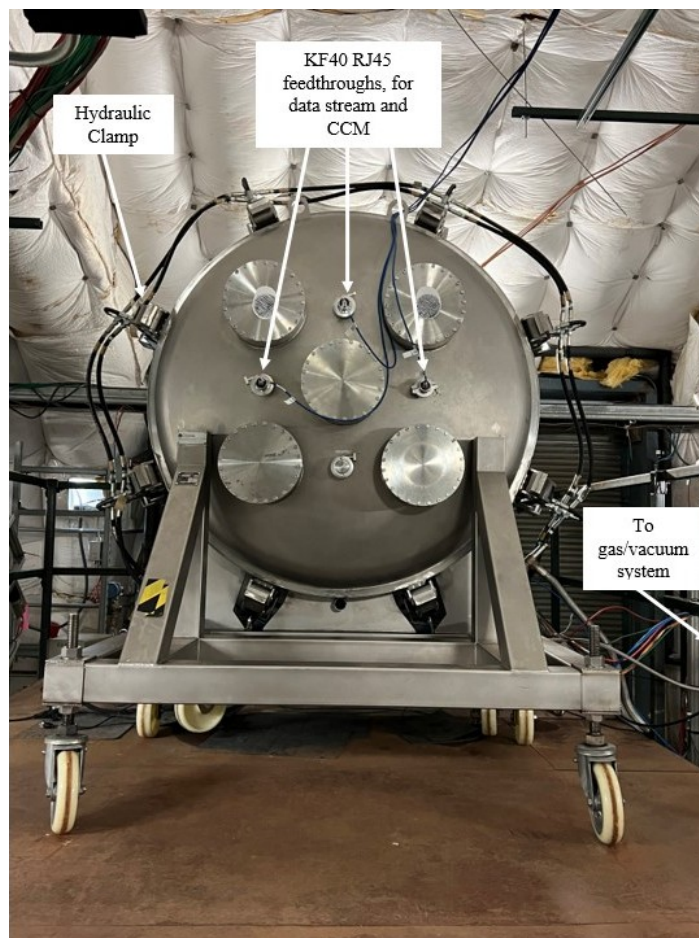
Figure 1. The TOAD pressure vessel in the test environment at Fermilab. Around the vessel, the hydraulic pressure clamps can be seen. In the centre, there is access to five flanges, which are unused in TOAD but previously used for mounting an optical readout system. The KF40 feedthroughs that are used for data readout and Control Configuration and Monitoring (CCM) via the blue cables are labelled. Various other KF40 and KF25 flanges on the vessel provide access for the different subsystems, but cannot be seen in this image. The gas and evacuation system is to the right of the vessel.
