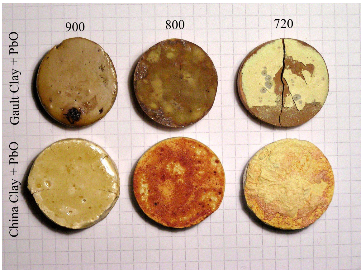
Figure 3.33: Gault and china clays glazed with PbO fired at 720, 800, and 900°C with dwell times of two hours. Note that each square of the above grid represents 1cm 2 .
