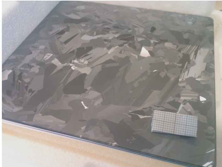
Figure 1.16: Multicrystalline silicon wafer, with 2 x 1cm bar for scale.
