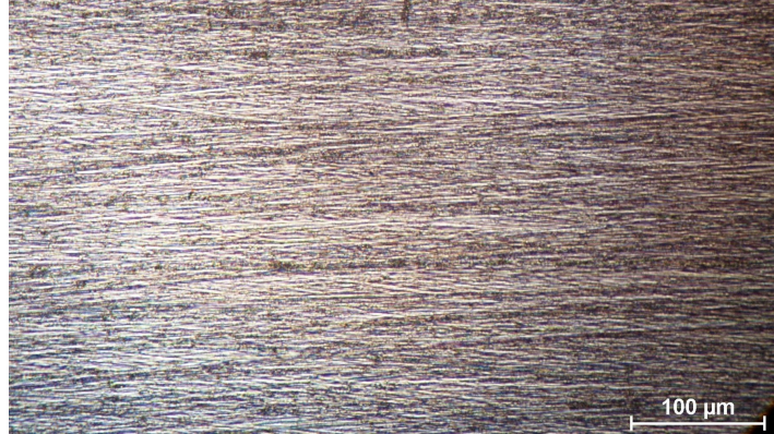
(a) Optical micrograph of silicon surface after P2500 grinding step.
