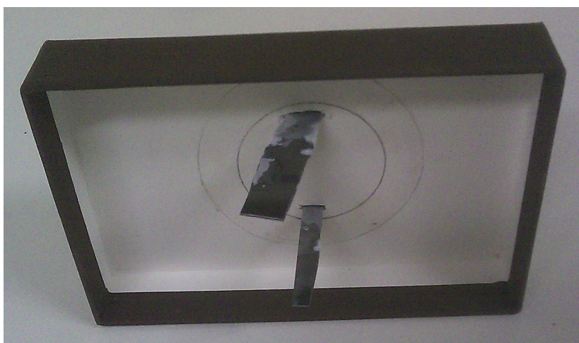
Figure 3.6: Photograph of reference and auxiliary electrodes and the frame used to secure them into the anodic etching cell.
