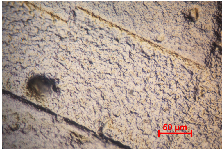
Figure 6.6: Optical micrograph of mc-Si anodically etched for 100 hours with no applied potential, showing rough surface texture.
