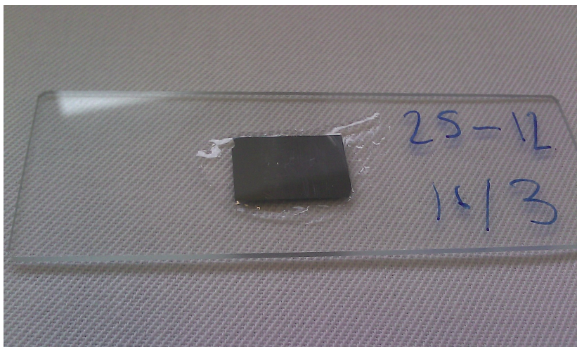
Figure 4.7: Etched and angle lapped mc-Si sample mounted on microscope slide.
