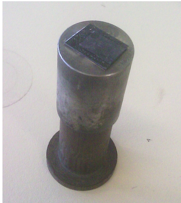
Figure 4.5: Photograph of flat stub showing handle and angled platform. Attached mc-Si sample measures 15 x 10mm.
