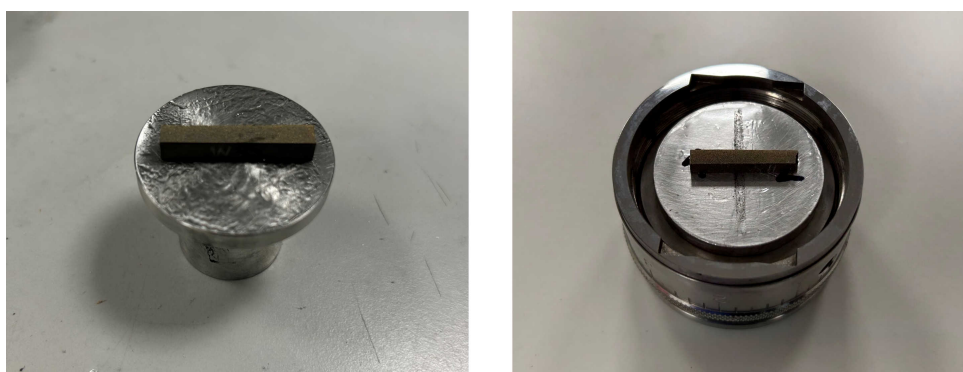
Fig. 5.44: Raw specimen mounted on the Al stub by using mounting wax (lhs), and stub screwed into the polishing frame (rhs).
