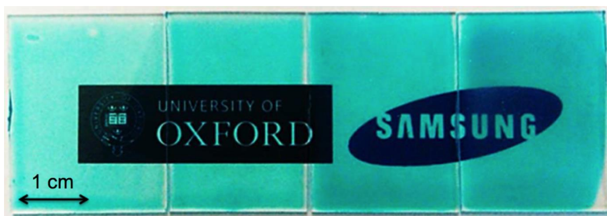
Figure 3.2 MOF thin films with increasing thickness, from left to right ca. 1, 2, 5 10 \mu\text{m} , obtained from sol-gel method of \text{G}\supset\text{DMSO} and deposited via doctor-blade technique. Film thicknesses were characterised by Alicona infinite focus microscopy using a 3D non-contact optical profilometer.
