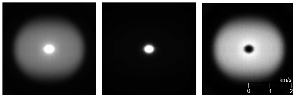
Figure 2.16: From left to right, a raw ion image of \text{HCl}(v' = 0, j' = 1) generated in a co-expanded mixture of \text{Cl}_2 and ethane, an image of the background HCl obtained without the photolysis laser firing, and the image obtained with the background subtracted.
