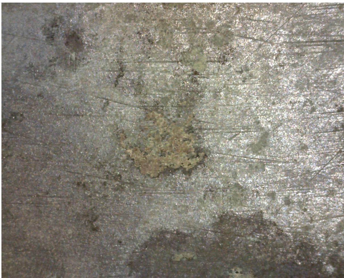
Figure 6.15 Striation marks partially covered by corrosion products (curved-spine knife 1945,1017.189) (author' photos)
