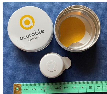
Figure 1 AcuPebble SA100 device (scale in centimetre). Image created by M A Miller.
