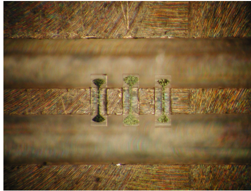
Figure 4.10: The LO directional waveguide coupler sitting in the shallow slot between the LO signal waveguide and the RF signal waveguide.
