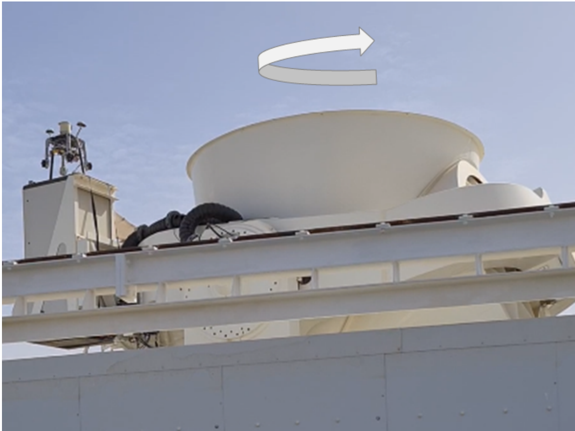
Figure 18. The UAV fastened on a rack cabinet alongside the telescope to acquire the azimuth rotation center.
