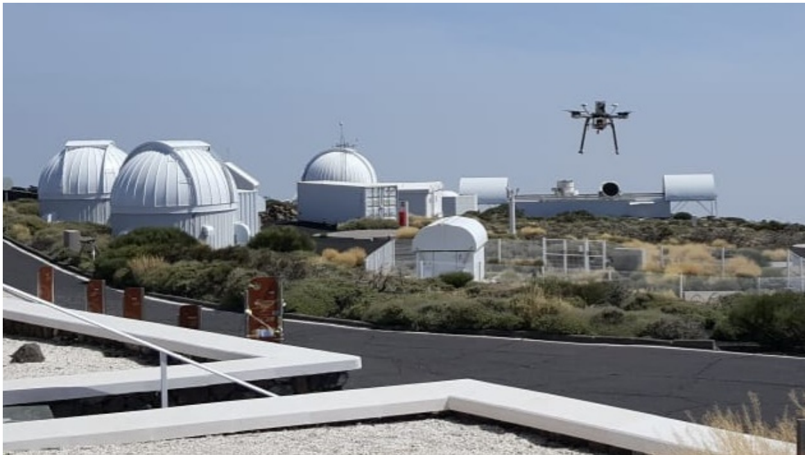
Figure 4. Photograph of the telescope and the UAV during the landing phase, taken near the home location. The black baffle of the second QUIJOTE telescope (the one on the right) is clearly visible beneath the UAV. The first QUIJOTE telescope is parked, pointing to zenith in the image.
