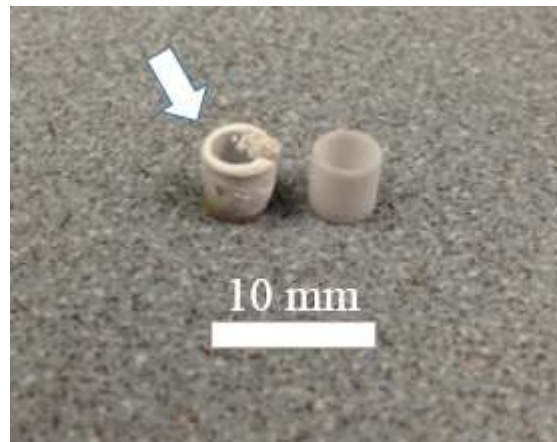
Figure 6.40 – Photograph showing that the walls of an alumina crucible were coated with MgO powder after a pure Mg sample was oxidized at 750°C for 1 h.
