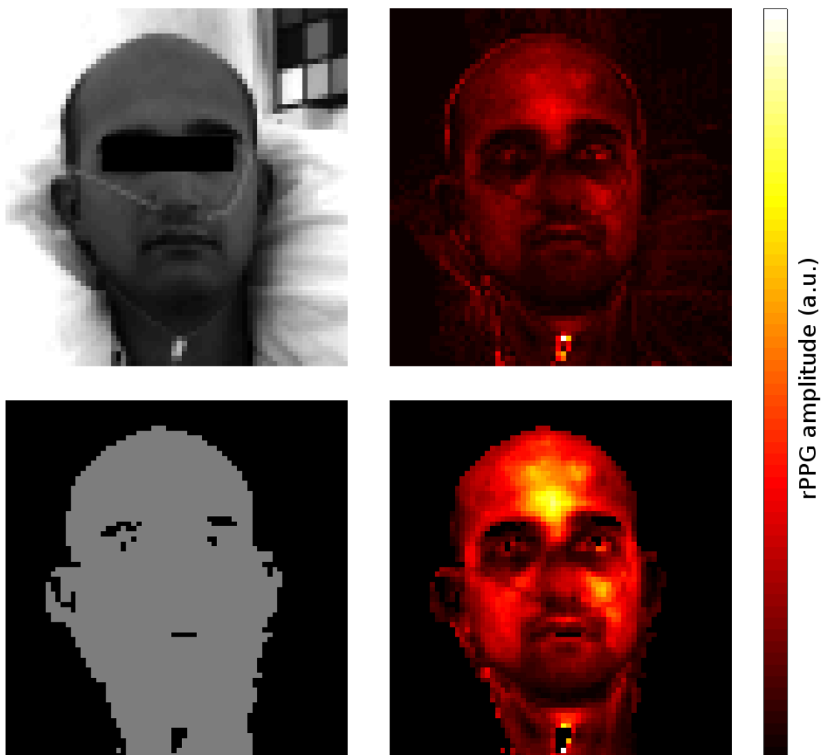
Figure 6.5: Example of mapping local rPPG amplitude in subject HP3-33 of the Physiology study. Top left: processed frame showing subject's position. Top right: raw amplitude map. Bottom left: mask showing areas identified as skin. Bottom right: processed amplitude map (after filtering and masking).
