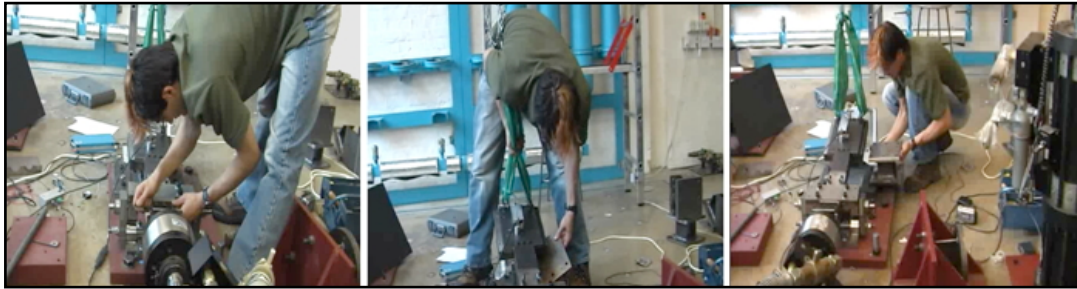
Fig 5. Disassembling the frame of a test rig and inserting a dissipative device.
