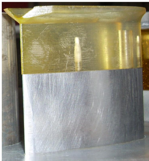
SI40 uncooled winglet tip on stainless steel base
