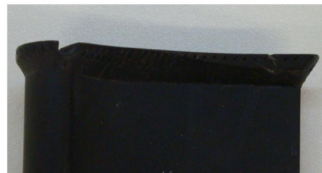
SI40 cooled winglet tip painted black for maximum IR emmissivity
