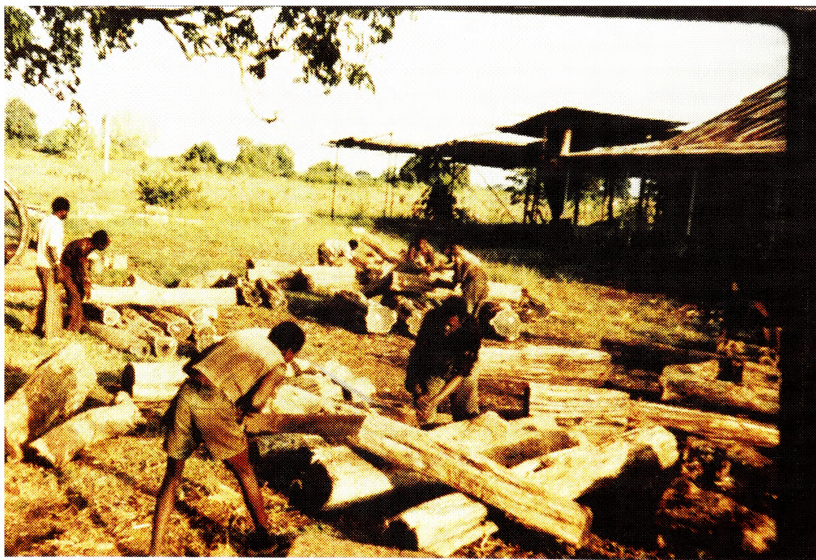
Appendix 2 Plate 11: Sawyer cross cutting Mpingo logs at E.A. Blackwood Enterprises - S.E. Tanzania.
