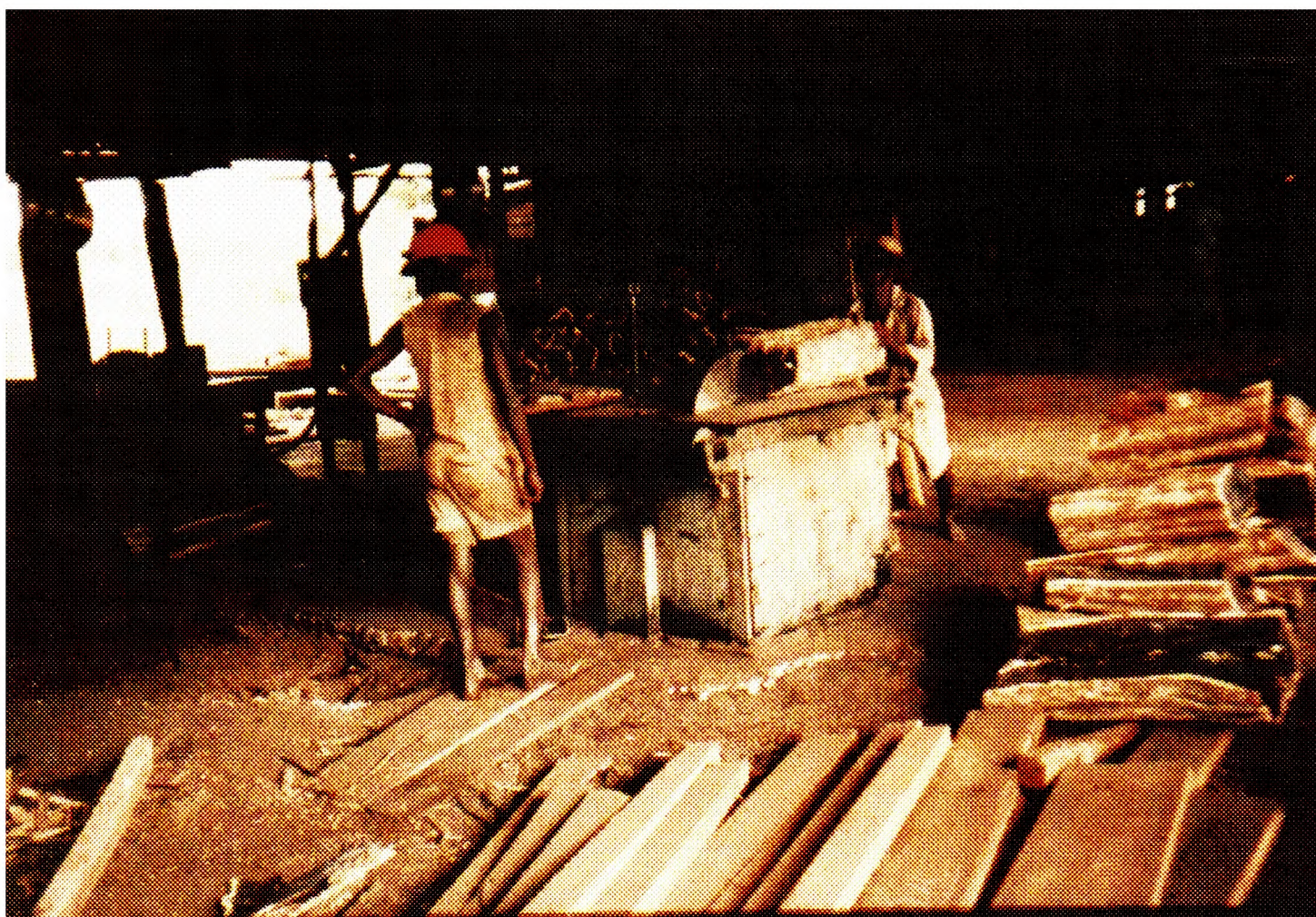
Appendix 2 Plate 10: Initial breakdown saw at Mingoyo Sawmill - S.E. Tanzania.
