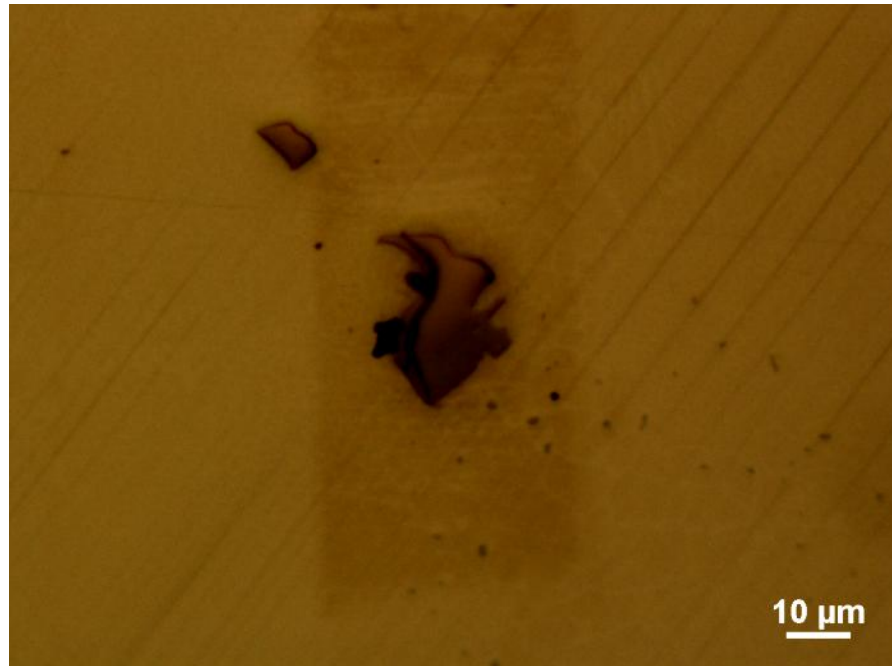
Figure 49. Optical micrograph of the carbide mapped in from sample 'P1' showing slip bands.
