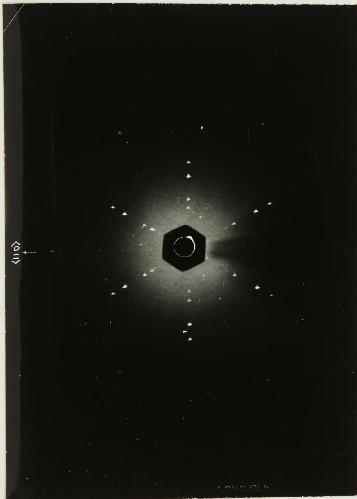
X-Ray Laue Photograph taken normal to an extracted \{111\} Irregular particle containing a \{111\} Spinel Twin
