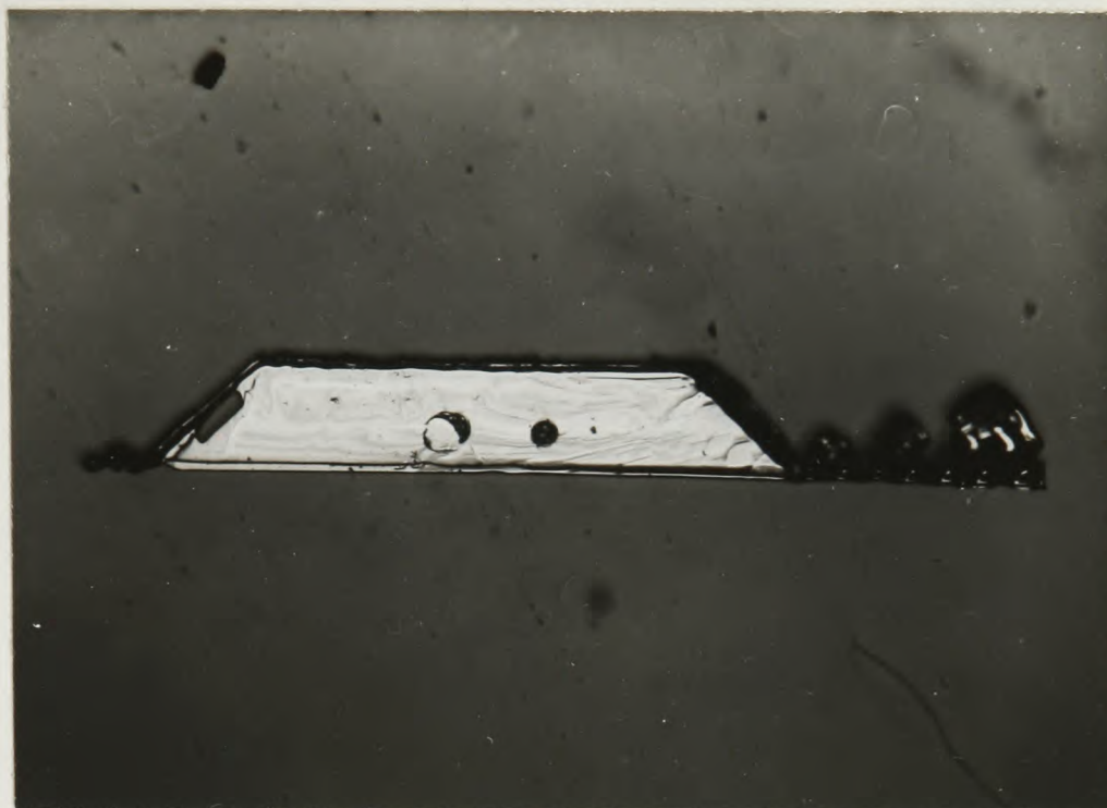
PLATE 47 Extracted Smooth Silicon Plate ( R = 1.54 \times 10^{-5} cm/sec. G \cong 30^\circ\text{C/cm.} )
