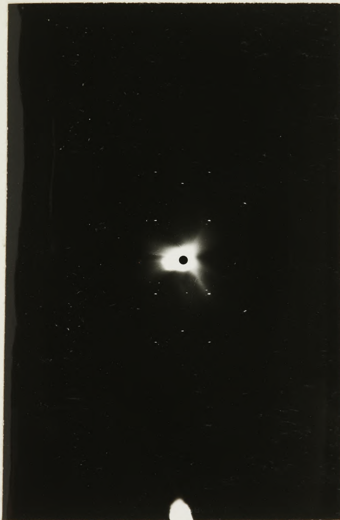
X-Ray Rotation Photograph (Cu K \alpha K \beta radiation) showing a \langle 110 \rangle Si preferred orientation
