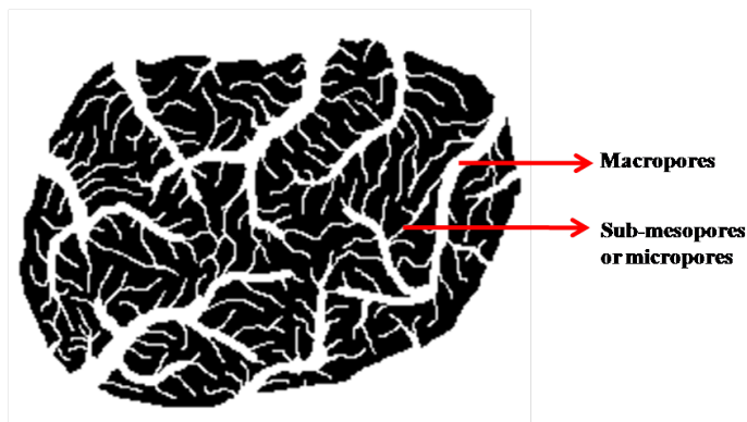
Figure 2.1: Schematic illustration of the inside porous structure of activated carbon particles.
