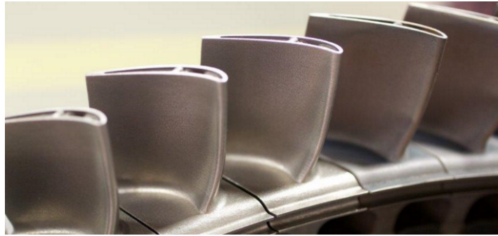
(b) Siemens 3D-printed tested blades [8]
