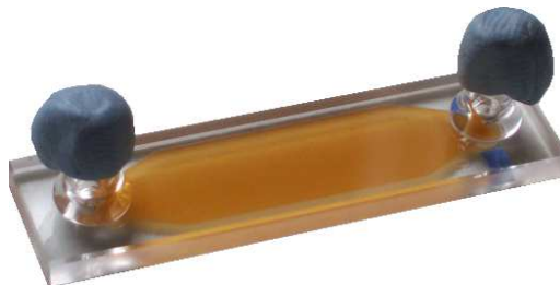
Figure 2.10: A Hellma sample cell containing 2.8 \mu\text{m} super-paramagnetic polystyrene colloidal particles. The colloidal particles are brown due to them containing iron oxide nanoparticles. The cell has length 45 mm, width 13 mm and internal height 200 \mu\text{m} . The inlet channels are sealed with Blu-tack.
