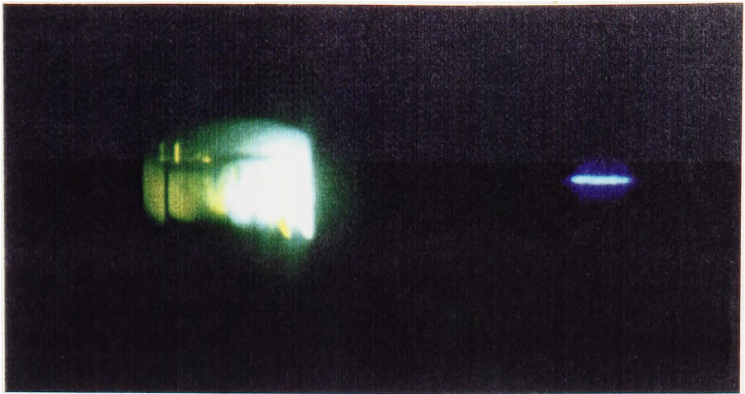
Plate VI-1. Dispersed harmonics. A piece of card in front of the power meter shows the fundamental beam and blue fluorescence from its second harmonic. By appropriate positioning of the recollimating lens, an image of the crystal is produced showing the path of the laser beam through the sample.
