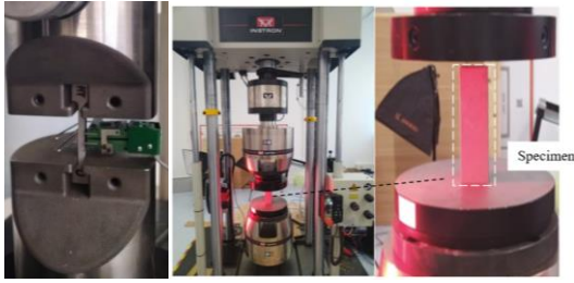
Figure 4 Tensile (left) and compression test set up (right)
