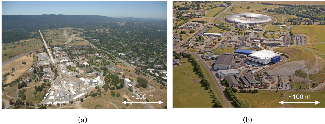
Figure 1.1: (a) Photograph of the SLAC National Accelerator Laboratory which operates a two-mile linear conventional accelerator, the housing of which can be identified by its linear, white roof. Photo courtesy of SLAC Linear Accelerator Laboratory. (b) Photograph of the Rutherford Appleton Laboratory (RAL) at which the Central Laser Facility (CLF) is situated. The Diamond Light Source, a synchrotron science facility, can be identified as a circular structure with a circumference of about 550m. Photo courtesy of Central Laser Facility.
