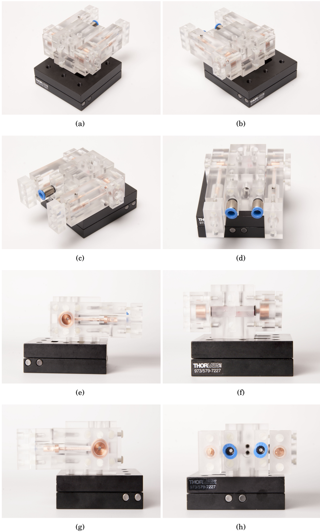
Figure 4.13: Photographs of the new housing on top of a Thorlab kinematic magnetic base.
