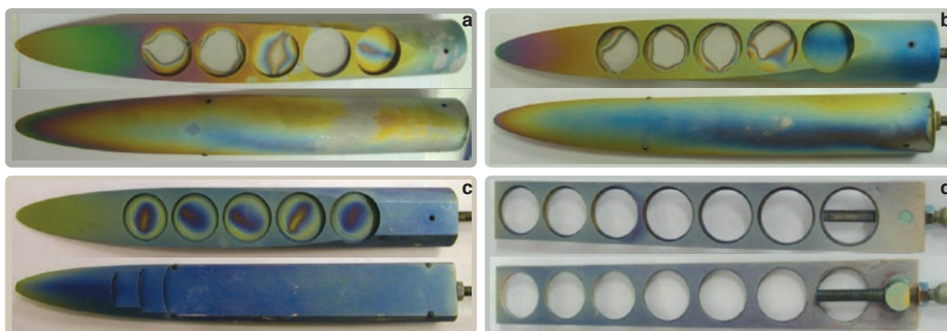
Figure 4.7: Top and bottom view of various sample holders that were coated with 300 ALD cycles of Zr_3N_4 . (a) beveled aluminum sample holder with 5 sec and (b) 10 sec long nitrogen purges at each ALD cycle. (c) beveled aluminum sample holder with less impedance to gas flow using 10 sec purge. (d) copper sample holder frame with very low gas flow impedance using 10 sec purge.
