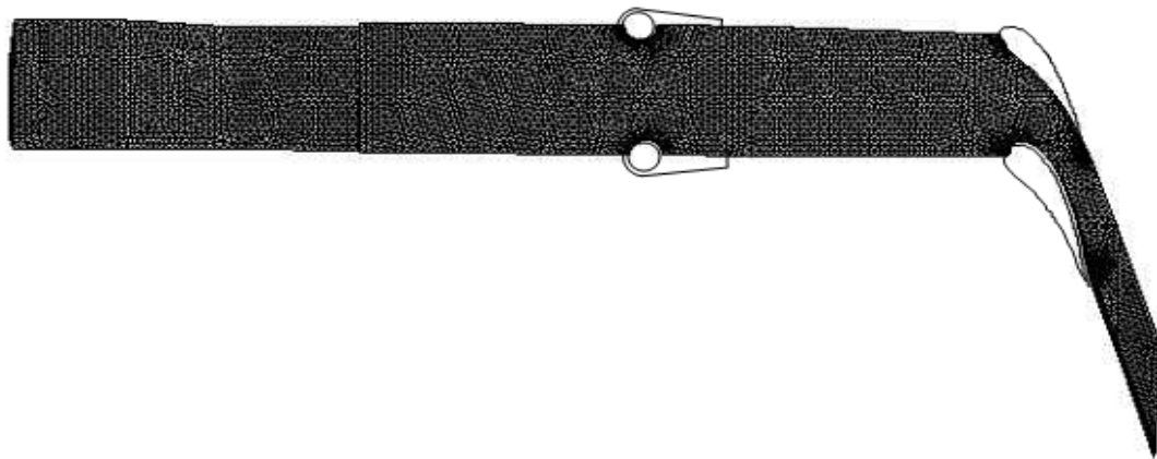
Figure 7.3: Span view of the assembled model of the combustor and vane passage with baffles and airfoil surfaces schematically present
