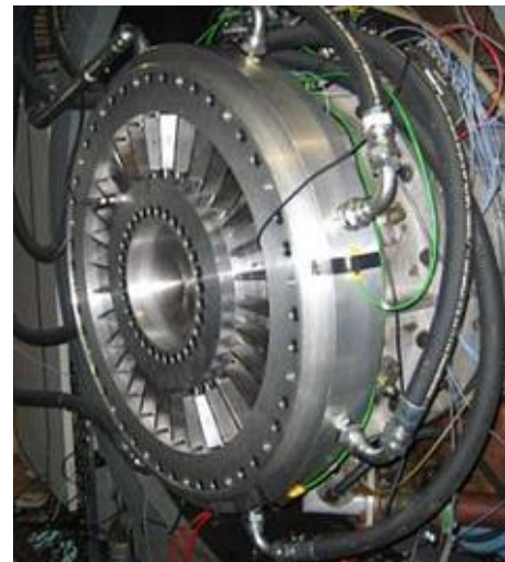
Figure 3.3: EOTDF module installed
