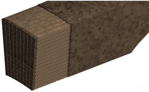
Figure 6.7: Mesh of the model with the tubes and constant area chamber
