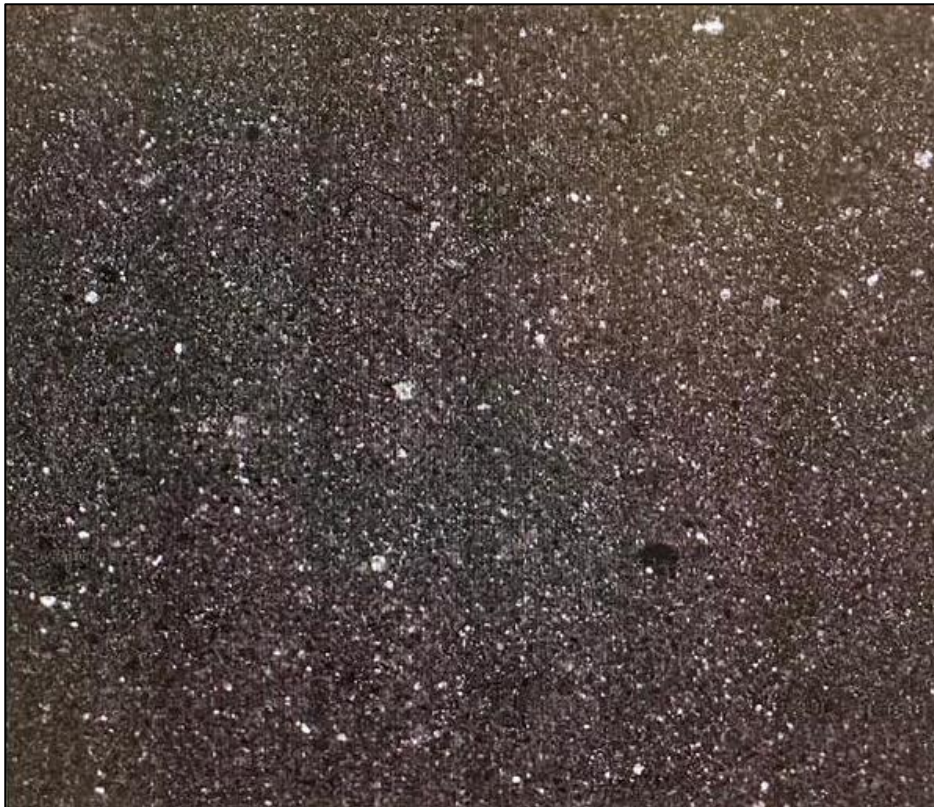
Figure 55: Showing a 10x10 mm 2D preview scan of an Apollo 11 (10084) sample which is ready to be profiled using the Alicona 3D ® non-contact surface profiler. The width of this square represents a third the width of the sample cup.
