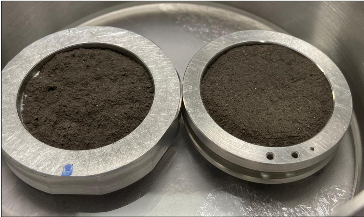
Figure 54: Left: a ‘rough’ Apollo 16 (68810) sample used in the VOSEG physical property variation study. Right: a ‘smooth’ Apollo 16 (68810) sample used in the VOSEG physical property variation study. Note, the inner diameter of the sample cup is 30 mm.
