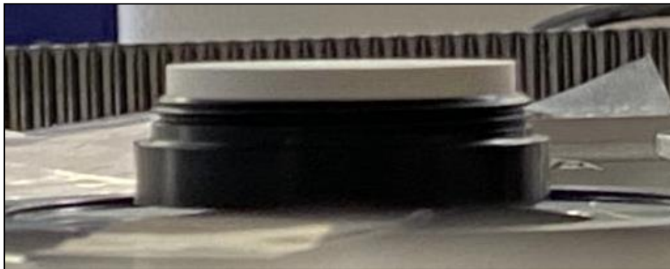
Figure 42: White Spectralon ® tilted ‘backwards’ (i.e. towards 0^\circ azimuthal angle) by 2.00 \pm 0.05^\circ .
