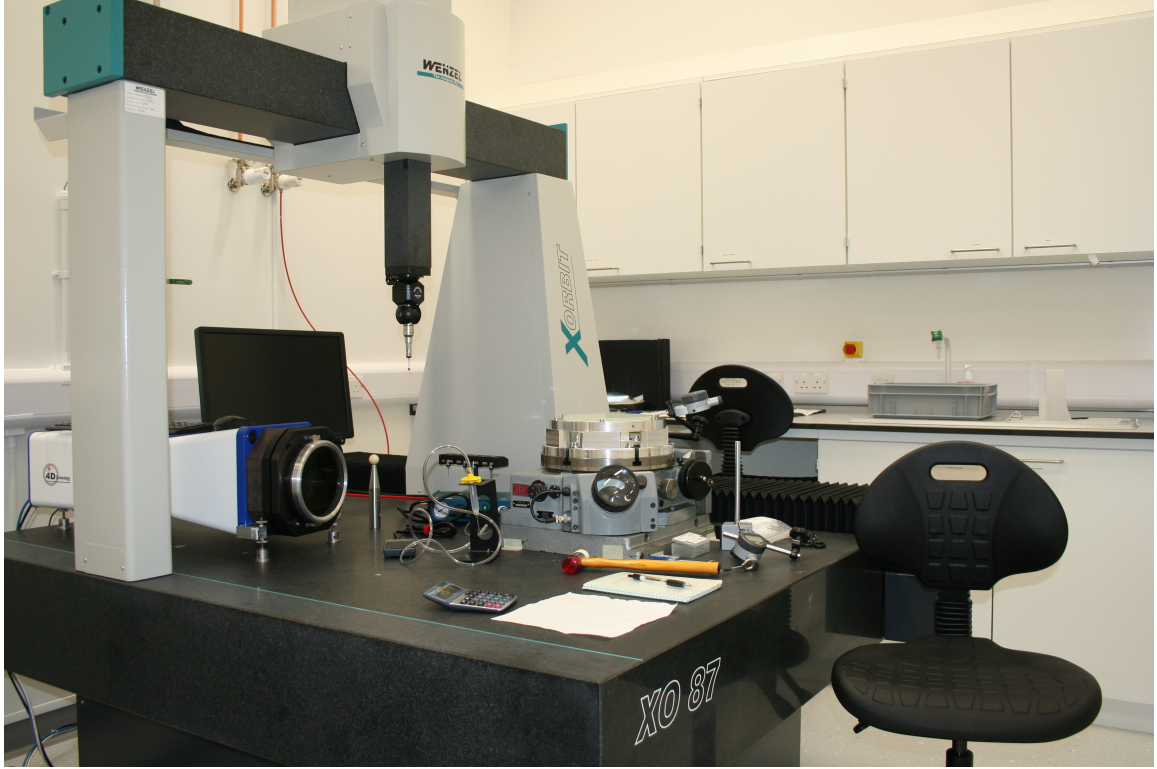
Figure 2.38: Coordinate measuring machine setup for measuring lens mount assemblies in cleanroom conditions at the instrument assembly lab in the University of Oxford. (Interferometer not used for this test.)
