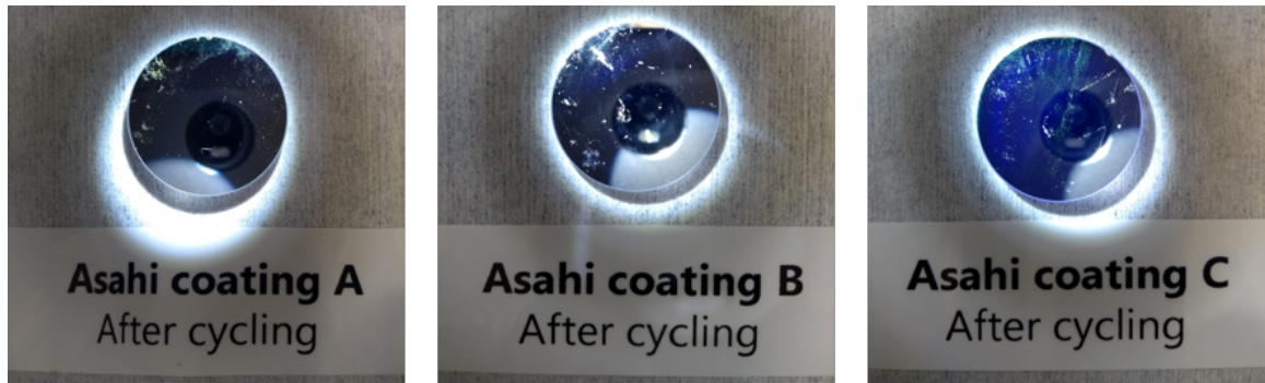
Figure 4.26: Asahi coating samples after being aged by thermal cycling.
