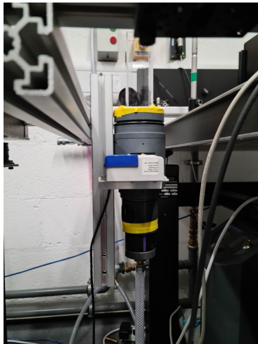
Figure 3.17: The laminar flow rig with vertical orientation.
