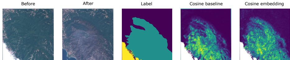
Figure 5: Additional comparison of the change detected using the baseline and the large VAE method on an example of a fire disaster. Both methods used a history of k = 3 frames. The cosine baseline prediction seems to more closely copy the details present in the image, making it susceptible to small, noisy variations between the two images.
