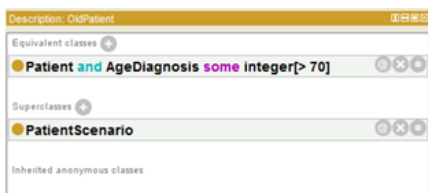
Figure 2.4: The ‘OldPatient’ defined OWL class with a ‘necessary and sufficient’ condition asserting its class equivalence. This entails that if something is a Patient and has a diagnosis age greater than 70, these conditions are sufficient to deduce that the OWL individual must be a member of the ‘OldPatient’ class.
