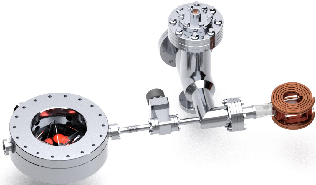
Figure 3.1: Schematic of the vacuum system. Atoms are first laser cooled in a pyramidal MOT (left) before transport to a UHV glass cell (right) using current-carrying coils mounted on a moving translation stage (not shown for clarity). Atoms are confined by a sequence of magnetic trapping potentials formed by static and RF fields produced by current-carrying coils (orange) which surround the UHV glass cell.
