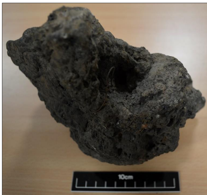
Plate 38, Impression caused by airflow into slag mass
