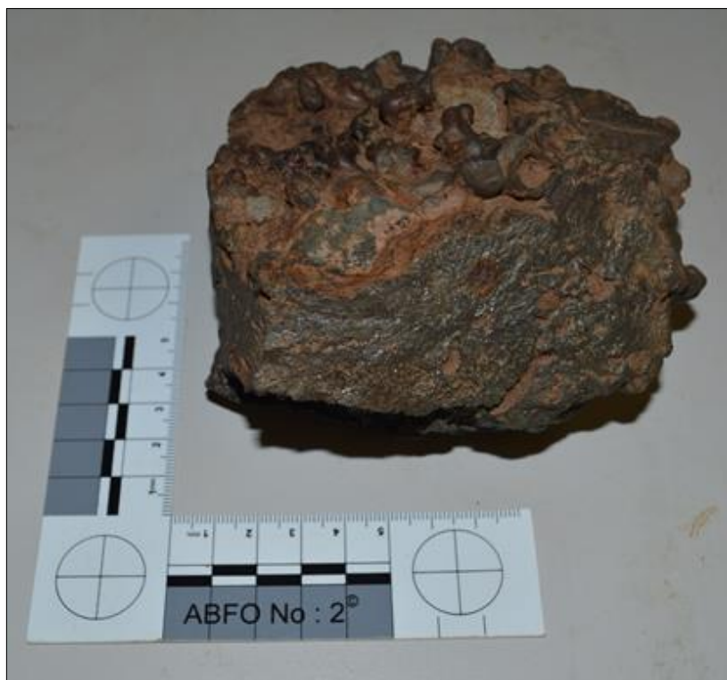
Plate 66, Dense furnace slag mass
