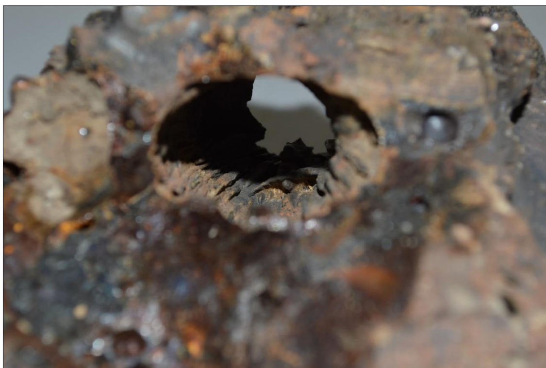
Plate 61, Airblast void in glassy mass (BP 4)
