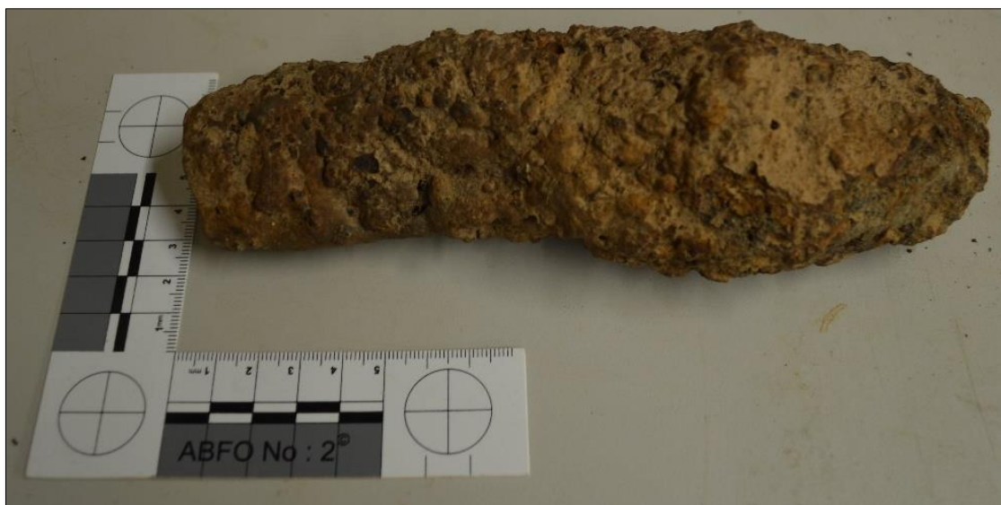
Plate 68, Slag tube with angled funnel end
