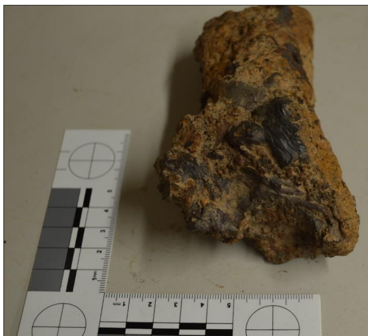
Plate 68, Slag tube with angled funnel end
